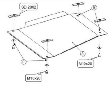
Fasten the part "3' with M 10x20 bolts and straps to the car frame. Tighten all screw joints.
