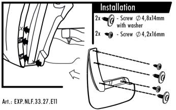
Set package  $\bigcirc$  Mudflap - 2 pcs; Spring clip - 4 pcs; Screw  $\bigcirc$  4,2x16mm - 4 pcs; Screw  $\bigcirc$  4,8x14mm - 4 pcs.
